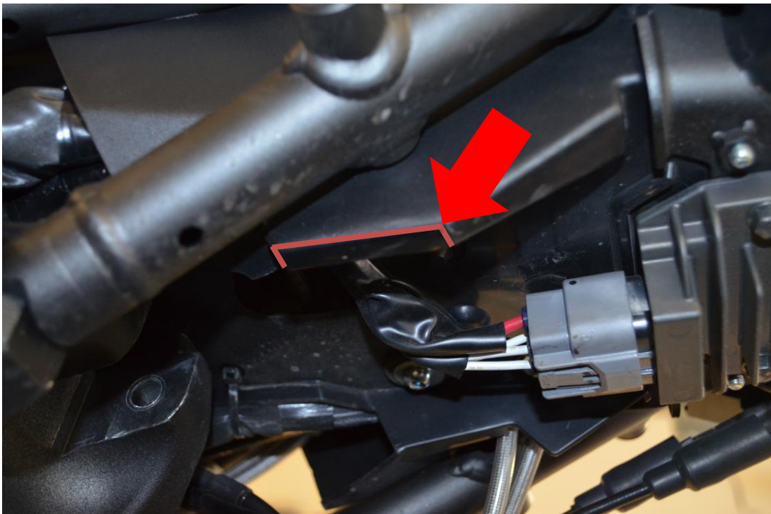
Figure 3: Undertray Edge to be Trimmed
