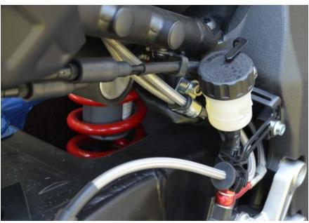
Be sure and check all lines for any binding or chafing when turning from left to right, or compression of the front and rear suspension. All Spiegler banjo fittings can be rotated per the instructions on the back of the inlay card to eliminate line twist and insure a proper installation.
